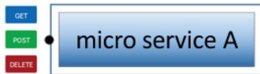
Figure 3: Schematic representation of a micro service providing a RESTful API wrapped in a Docker container.
